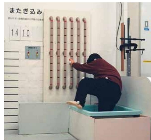
Experiments of simulated bathtub use with handrails in Japan (© Satoshi Kose)
